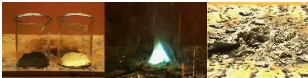
Figure 5.YY. Zinc and sulfur (a) react (b) to form zinc sulfide (c)
