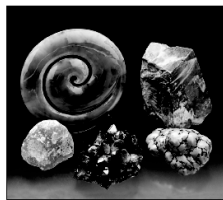
(c) Traces of transition metal ions are responsible for the colors in purple amethyst (iron), green jade (iron), red corundum (chromium), and blue lapis lazuli and turquoise (copper).
