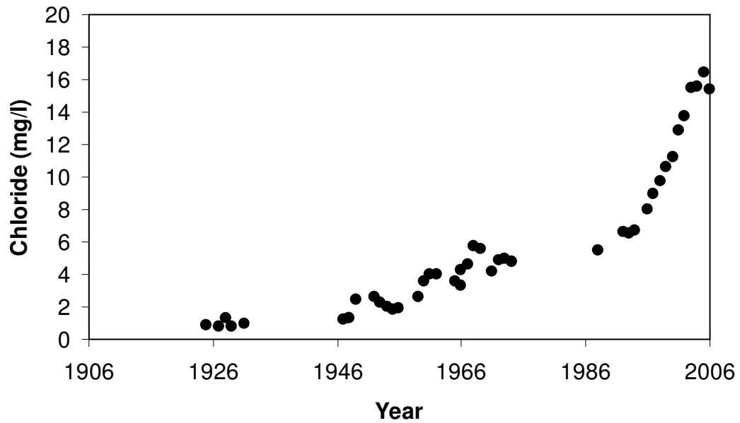
Figure 3. Mean chloride concentrations at TR4-C, 1925-2006. Points later than 1990 represent yearly averages (modified from Peters 1974).
